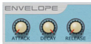
Note that "Transparent" function "obeys" the ADR envelope, so a slow attack, decay or release will cause the transparent audio to fade rather than instantly disappearing.
