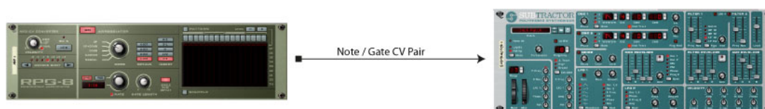
Fig. 1-2a: A typical Note / Gate (or CV / Gate) connection between a sequencer and an instrument
